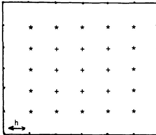
Figure 2.1. The uniform discretization of  $R$ .
